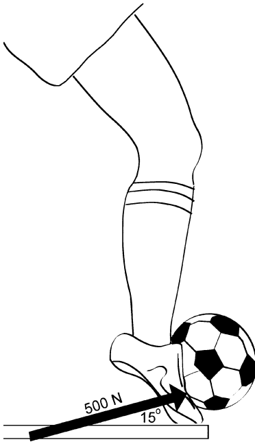
Figure 2.3. Vector representation of the force applied by a foot to a soccer ball. The magnitude and direction properties of a vector are both apparent on the diagram: the length of the arrow represents 500 Newtons of force, while the orientation and tip of the arrow represent the direction ( 15^\circ above horizontal) of the force.
